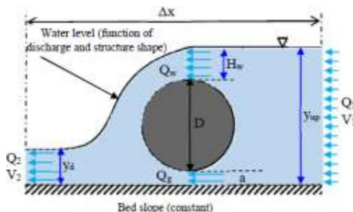
Fig. 1. Schematic diagram of combined over-under flows through a cylindrical weir-gate.
