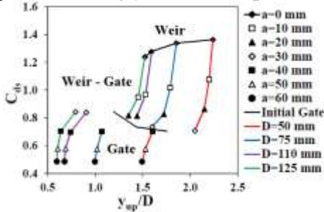
Fig. 4.  $C_{ds}$  versus  $[y_{up}/D]$  for discharge 14 Lit/sec
