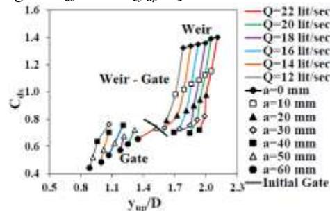
Fig. 6.  $C_{ds}$  versus  $[y_{up}/D]$  for Diameter 75 mm
