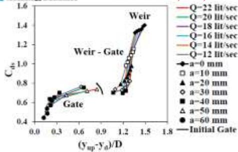
Fig. 10.  $C_{ds}$  versus  $[(y_{up}-y_d)/D]$  for Diameter 75 mm
