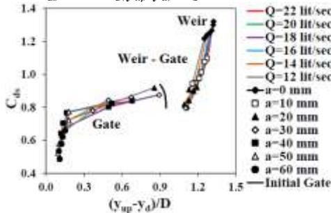
Fig. 12.  $C_{ds}$  versus  $[(y_{up}-y_d)/D]$  for Diameter 125 mm
