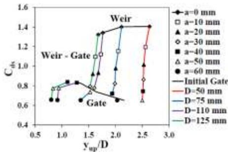
Fig. 2.  $C_{ds}$  versus  $[y_{up}/D]$  for discharge 22 Lit/sec
