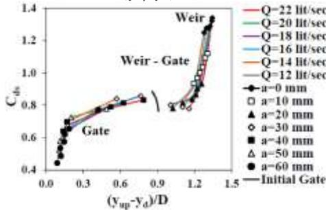
Fig. 11.  $C_{ds}$  versus  $[(y_{up}-y_d)/D]$  for Diameter 110 mm
