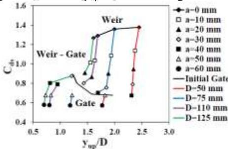
Fig. 3.  $C_{ds}$  versus  $[y_{up}/D]$  for discharge 18 Lit/sec
