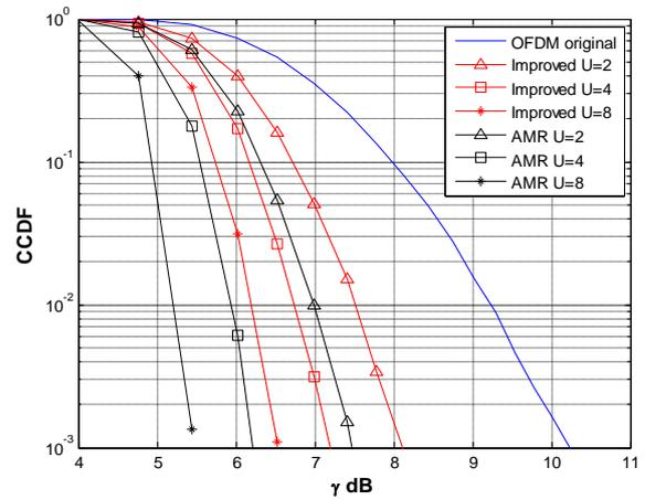
Figure 2 PAPR comparison for original SLM, Improved SLM and AMR SLM
