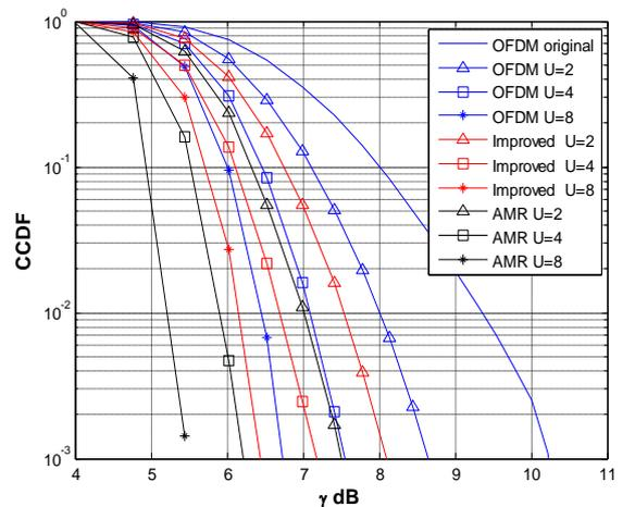
Figure 4 PAPR comparison for original SLM, Improved SLM and AMR SLM
